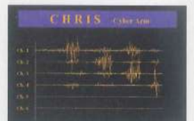
EMG信号を利用した手動制御型人間支援マニピュレータ。腕に貼った6つの電極が筋電を検知し、義手ロボットが腕と同時に動く。上は筋電測定画面。Human assisting manipulator operated by EMG signals. Six electrodes attached to the operator's arm detect EMG signals and the prosthetic moves in sync with the operator's arm.
