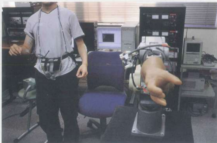
EMG信号を利用した手動制御型人間支援マニピュレータ。腕に貼った6つの電極が筋電を検知し、義手ロボットが腕と同時に動く。上は筋電測定画面。Human assisting manipulator operated by EMG signals. Six electrodes attached to the operator's arm detect EMG signals and the prosthetic moves in sync with the operator's arm.
