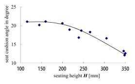
Figure 10. The relationship between seat cushion angle and H for passenger cars in stock
