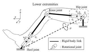
Figure 12. The rigid link model for computation
