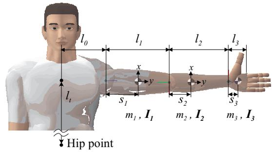
Figure 5: A multibody human model of upper extremity.
