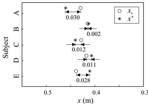
Figure 7: Comparison between optimized and ergonomically comfort longitudinal position of the steering wheel.
