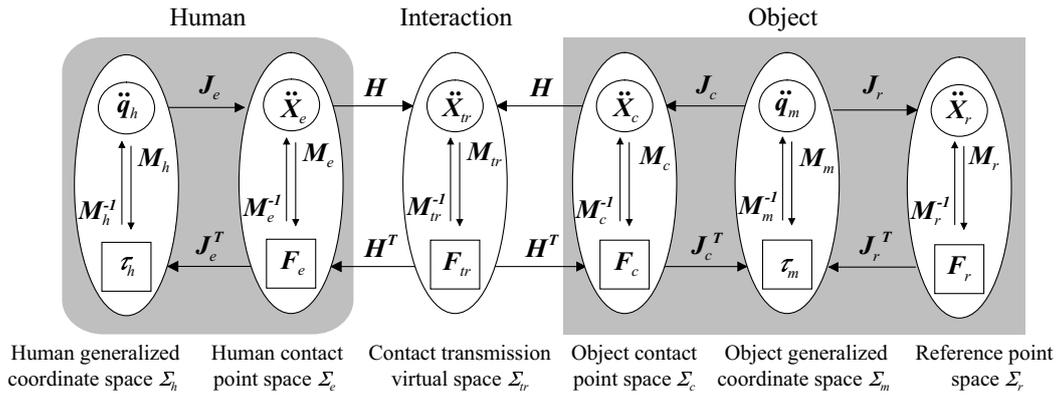
Figure 2: Force/acceleration relationships in a human-machine system [5]
