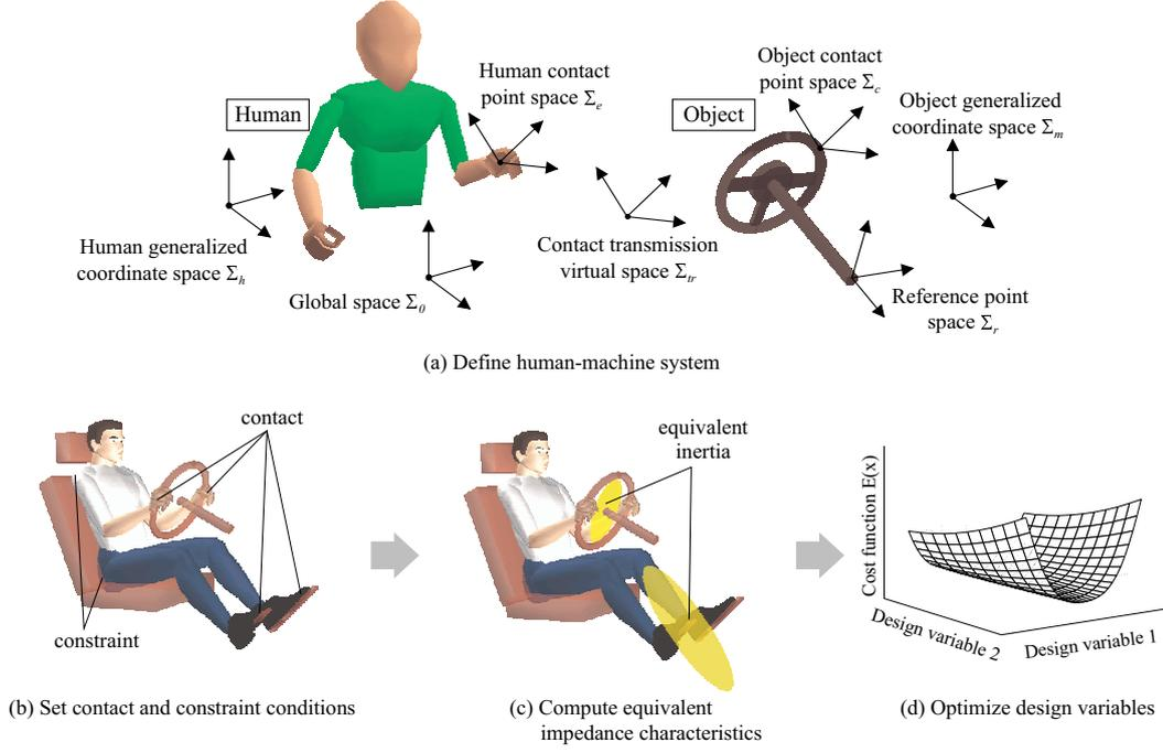
Figure 1: Framework of the proposed layout design method based on equivalent inertia of human-machine systems.
