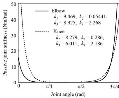
Figure 6: Joint passive stiffness of elbow and knee joint.
