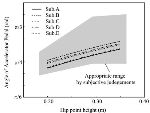
Figure 10: Effective equivalent inertia angle and appropriate range of accelerator angle.
