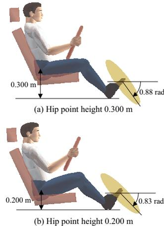
Figure 9: Examples of effective equivalent inertia angle.
