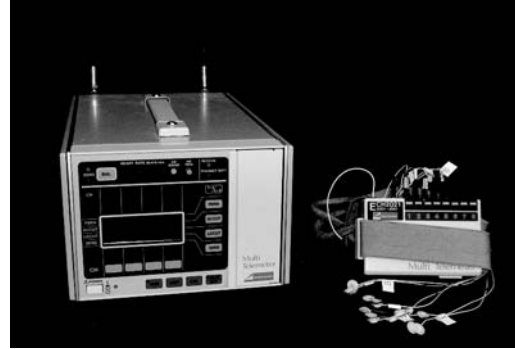
Figure 5. The multi-telemeter (Web5000) and electrodes (NT-511G) used in the experiments
