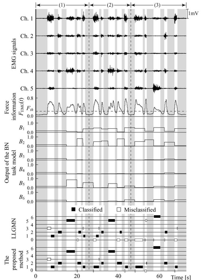
Fig. 11. Sample session of experimental results of a manipulation trial (task of taking meal; subject A). The labels of classification results are as follows: 0—Decision suspension (no motion command is generated for the manipulator), 1—hand open, 2—hand grasp, 3—flexion, 4—extension, 5—pronation, and 6—supination.
