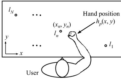
Fig. 2. Locations and the user's hand position in the workspace. Location of motion is determined according to coordinates of hand position.
