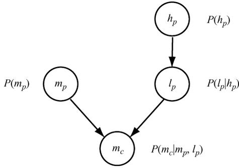
Fig. 1. Task model for motion prediction using a BN.
