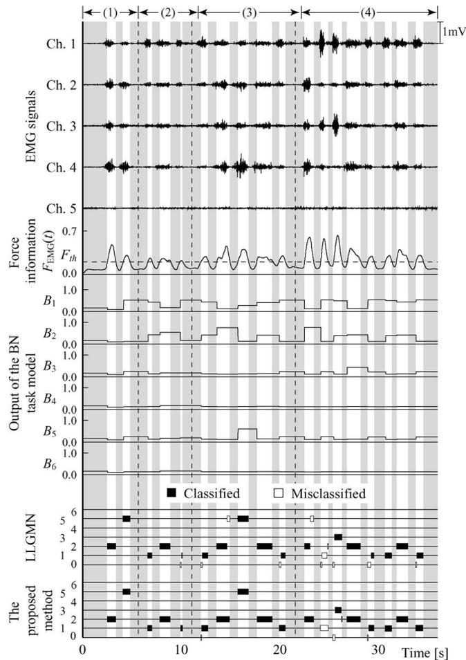
Fig. 5. Example of continuous classification results of the cooking task (subject A). The labels of classification results are as follows: 0—Decision suspension, 1—hand open, 2—hand grasp, 3—flexion, 4—extension, 5—pronation, and 6—supination.
