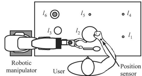
Fig. 10. Workspace of the task of taking meal. A robotic manipulator is set on the left side. The items in the workspace are a disk and a spoon ( $l_2$ ), a glass ( $l_3$ ), and a bottle of water ( $l_6$ ).
