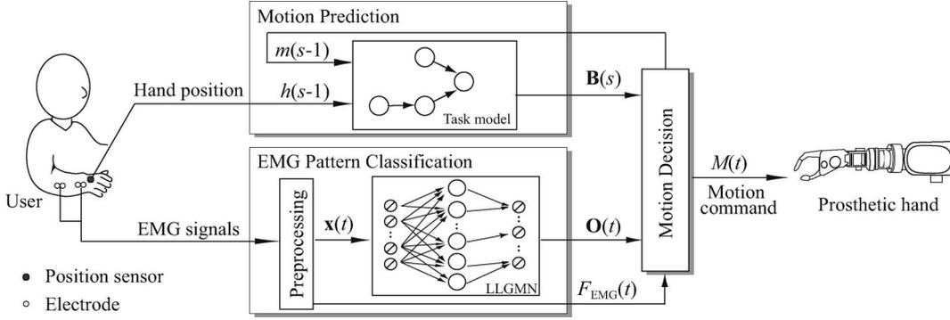
Fig. 3. Hybrid structure of an EMG-based human-robot interface, where the BN task model is incorporated for motion prediction.
