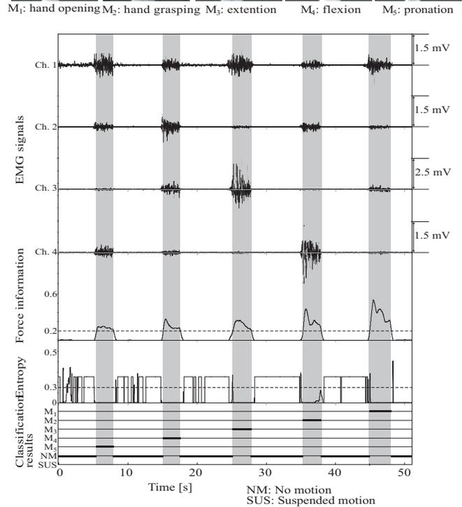
Fig. 7. Examples of measured EMG signals and classification results (Subject A)
