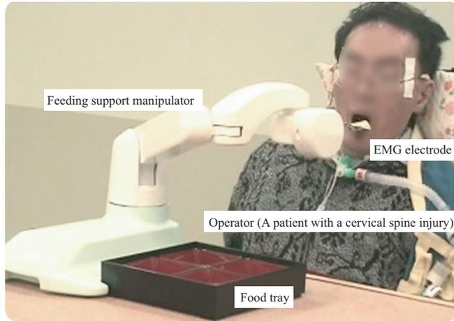
Fig. 2. Example of feeding support manipulator operation by a patient with a cervical spine injury
