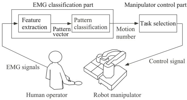
Fig. 1. System components of the mealtime support manipulator
