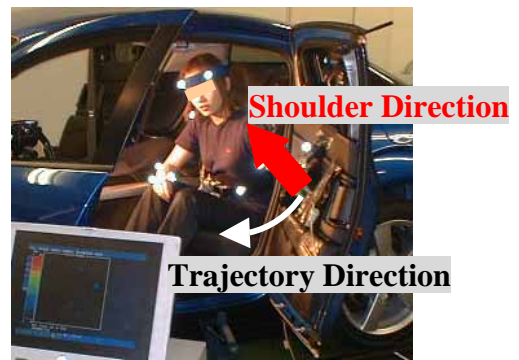
Fig.20 Door Operation Test
