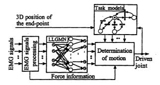
Figure 1: Structure of the proposed method.
